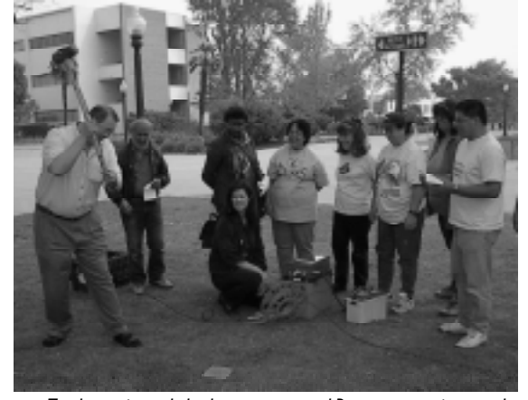
Teachers using a sledge hammer to record P-waves on a seismograph.
